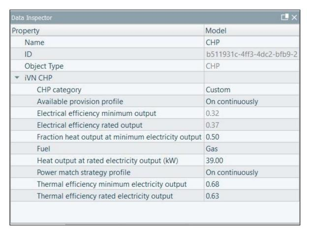
(Image shows and example of a CHP asset parameters)
