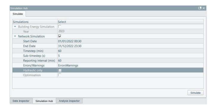
The hydraulic model is used for computing the flow rate and pressure head for each pipe. iVN uses the nodal method in combination with demand-driven analysis to assume a steady-state solution. This involves the solution of the Bernoulli equation considering flow rate boundary conditions and head losses in pipes due to friction - but as water is assumed to be incompressible and its properties are temperature invariant, the problem becomes framed in terms of volume flow rate.
